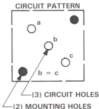
NOTE: THIS ELEMENT CAN BE ROTATED 180° SO POSITION a, b, c BECOMES c, b, a.
